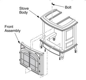
Figure 13 - Removing Front Assembly (Oxford™ Model Shown)
